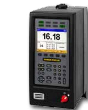
By using torque monitoring control combined with angle control to measure degrees of rotation from the point of tool engagement in the workpiece, the Tensor S system enables the user to tap to a precise depth.
