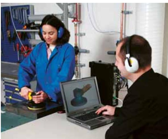
Atlas Copco has a well equipped laboratory for measuring tool noise and vibration emissions. It contains advanced vibration measurement tools, a state-of-the-art acoustics laboratory and dedicated computer software for analysing measurement and test results.
